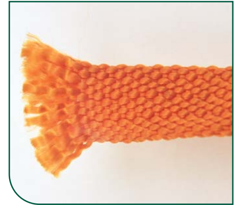
Figure 12.2 Cut, damaged yarn
