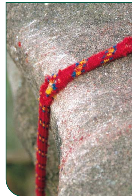
Figure 10.3 Serious damage to a rope in use
