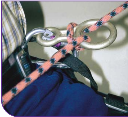
Figure 1.3 A figure-of-8 forcing open a screwgate karabiner. Photo: BMC Collection
