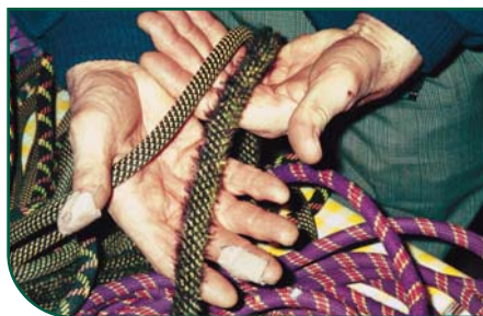
Figure 10.4 Furry, over-used ropes Photo: BMC Collection
