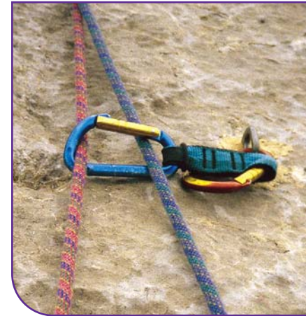
Figure 1.5 Badly-positioned karabiner Photo: George Steele
