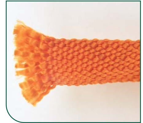
Figure 12.2 Cut, damaged yarn
