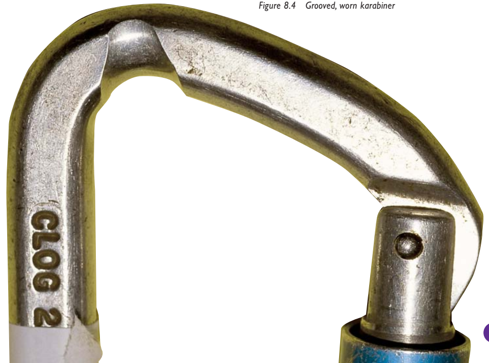
Figure 8.4 Grooved, worn karabiner
