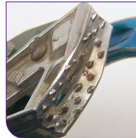
Figure 6.4 Ascender with worn and damaged teeth
